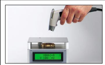
Figure 9. Charge Plate Monitor and Static Decay Time Measurements using <u>980/980E</u> Air Gun Ionizer.
