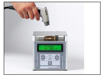
Figure 8. SCS <u>711</u> Charge Analyzer Static Decay Time and Balance Operation.
