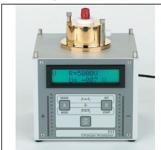
Figure 4. SCS <u>711</u> Charge Analyzer Voltmeter Operation.
