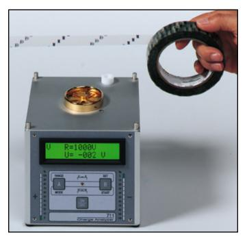
Figure 3. Testing Low Tribocharging Tapes.
