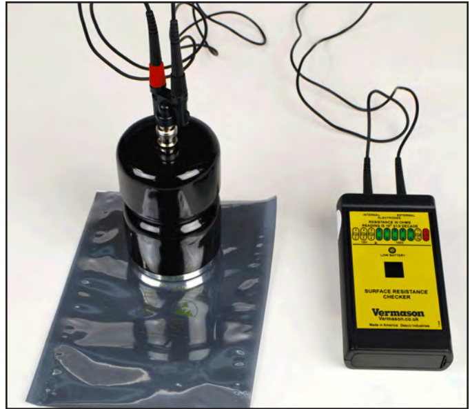
Figure 5. Using the Concentric Ring Probe with the Vermason Surface Resistance Checker
