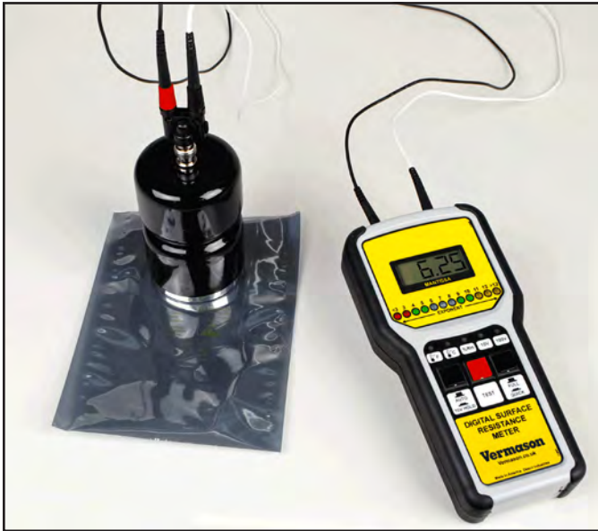
Figure 3. Using the Concentric Ring Probe with the Vermason Digital Surface Resistance Meter
