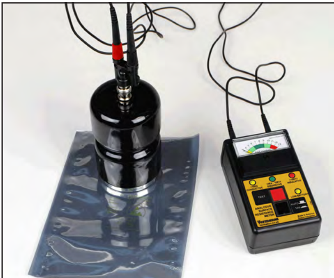
Figure 4. Using the Concentric Ring Probe with the Vermason Analogue Surface Resistance Meter
