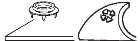
Figure 9. Installing push and clinch mat grounding snap.
