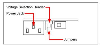
Figure 5. 220V jumper setting
