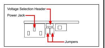
Figure 4. 110V jumper setting
